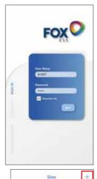
Step 2: Press the '+' icon on the homepage to add plant. Press the scan icon next to the 'Datalogger List' to scan the QR code label on front side of the Smart WiFi.
